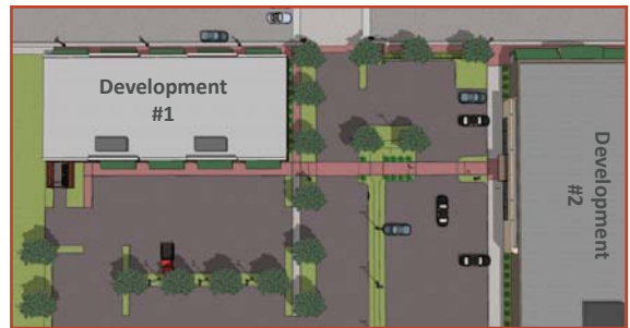
This illustration shows two developments on adjoining lots sharing parking and an access drive. A sidewalk connects the two developments through the parking area.
