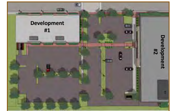
This illustration shows two developments on adjoining lots sharing parking and an access drive. A sidewalk connects the two developments through the parking area.
