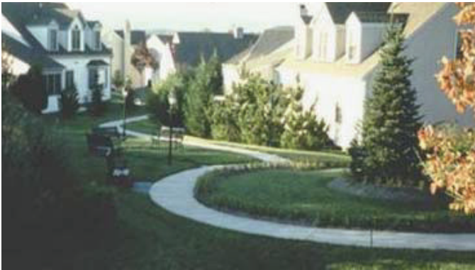
Sidewalk that drains to adjacent vegetation and provides common walkways linking pedestrian areas.
